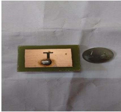
Figure.3.8: Fabricated T-Slot Loaded Rectangular Microstrip Patch Radiating Patch.
