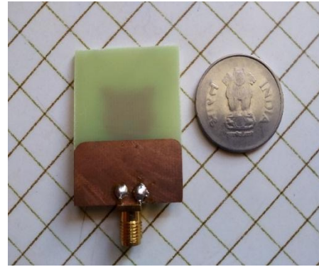
Figure.3.45: Fabricated Slotted Key Shape Monopole Rectangular Microstrip Patch Antenna with Rounded Corner in Partial Ground, Ground Plane
