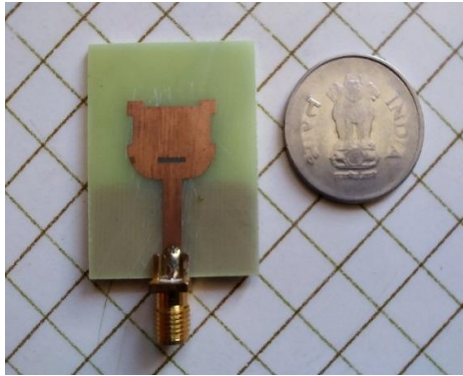
Figure.3.44: Fabricated Slotted Key Shape Monopole Rectangular Microstrip Patch Antenna with Rounded Corner in Partial Ground Radiating Patch
