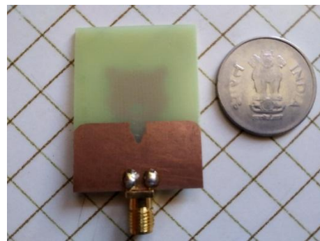
Figure. 3.51: Fabricated Key Shape oval slotted monopole Rectangular Microstrip Patch with rounded corner and groove shaped notch in partial ground, ground plane
