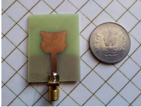
Figure.3.40: Fabricated Key Shape Rectangular Microstrip Patch with Rounded Corner in Partial Ground Radiating Patch.
