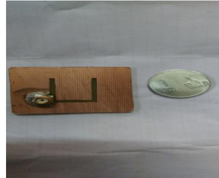
Figure. 3.7 Fabricated U-Slot with Defective Ground Structure (DGS) Ground Plane.
