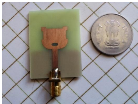
Figure. 3.50: Fabricated Key Shape oval slotted monopole Rectangular Microstrip Patch with rounded corner and groove shaped notch in partial ground radiating patch
